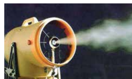
Portable fogging machines can be utilised with various propellants to disperse fungicides and insecticides in green houses
