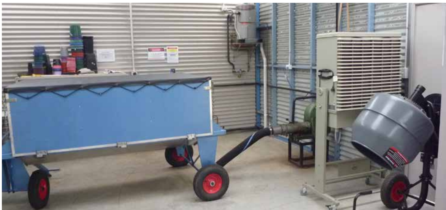
A steam sterilising unit at Great Southern IT – WA (NIASA Accredited)
