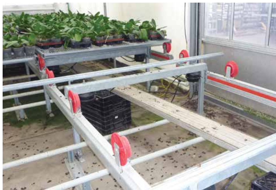
Another use of gas is demonstrated in the use of a compressed air bench lifter to assist with the rotation of stock in a glass house (Jong's Nursery South Australia)
