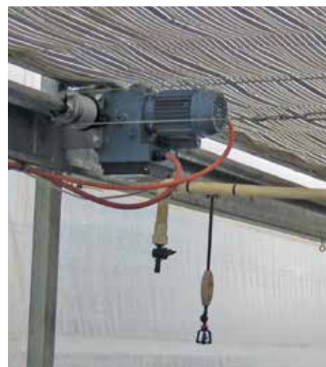
Internal screens used to reduce light and thermal energy (day) to modify the greenhouse environment and retracted at night for heat retention. NIASA accredited Alstonville Palms NSW.
