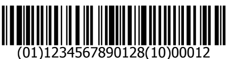
An example of a GS1-128 barcode with a GTIN and a batch number. Note the Application Identifiers in brackets.
