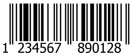
An example of an EAN-13 barcode encoding a GTIN
