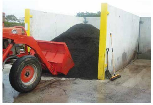
Fig #1 – A concrete storage area is ideal, with a large concrete apron leading up to the bay(s). This nursery also employs the use of a dedicated bucket/shovel just for media, otherwise, they should be regularly disinfested. Clyde Plant Nursery
