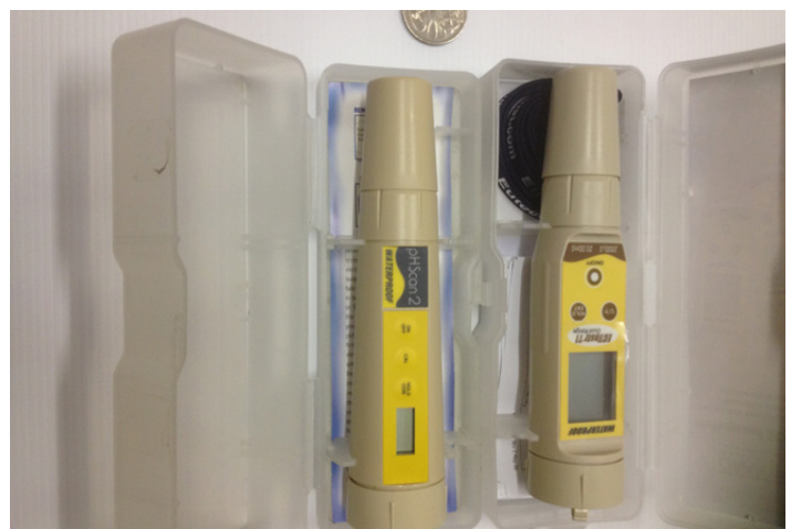
Portable pH and EC meters are a convenient way to monitor basic chemical properties of irrigation water in the field looking for changes in water quality.
