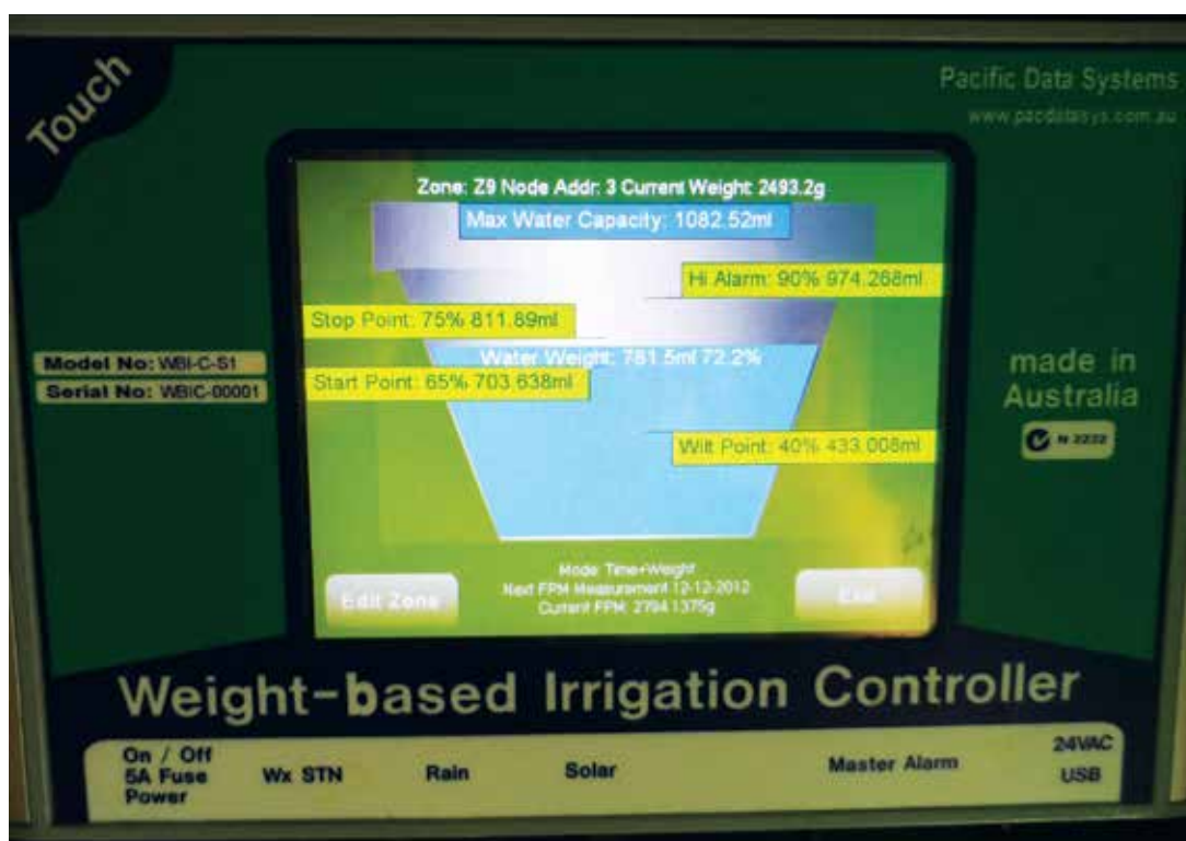
Figure 7: WBIC Touch Screen – diagrammatic view for setting Stop Point, Start Point, Wilt Point and over irrigation alarm point.
