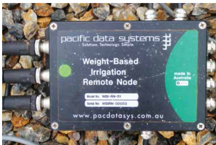
Figure 3: An in-field WBIC network node for connection solenoids, weighing devices and other sensors
