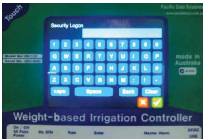
Figure 6: WBIC unit with touch screen interface and security logon screen
