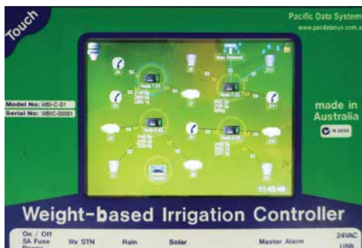
Figure 4: WBIC unit with touch screen interface
