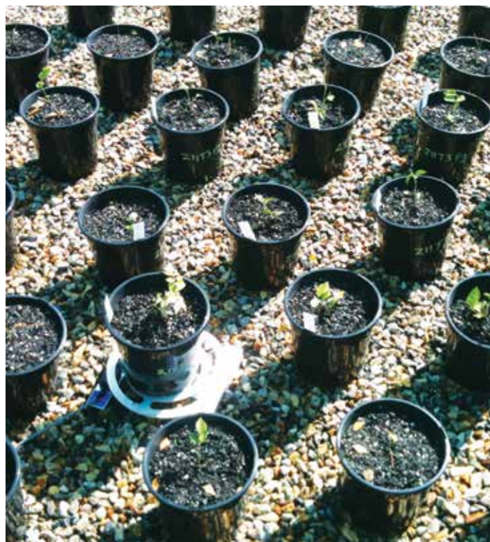
Figure 5: Loadcell used to monitor plant weights and trigger irrigations
