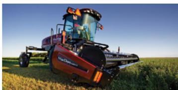
A new windrower has helped a family business in Ballarat, Victoria reduce diesel consumption by about 25 per cent, cut carbon emissions and improve energy productivity. The windrower saves 2 to 2.5 litres of diesel per hectare.
